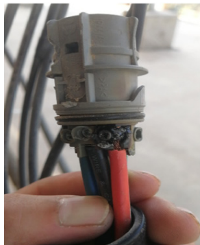
Insufficient contact and crimping of the conductor increase the risk of virtual connection
