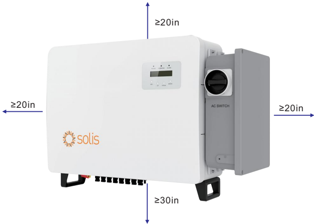
Figure 3.2 Clearance distances requirement for the inverter
