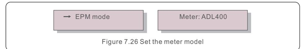
Figure 7.26 Set the meter model
