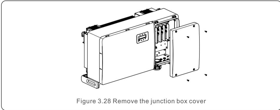
Figure 3.28 Remove the junction box cover
