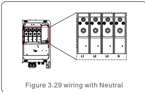
Figure 3.29 wiring with Neutral
