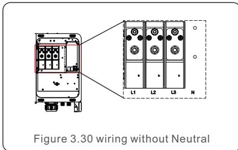
Figure 3.30 wiring without Neutral
