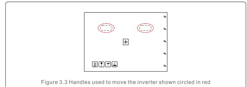
2. Two people are required to remove the inverter from the shipping box. Use the handles integrated into the heat sink to remove the inverter from the carton (see Figure 3.4).
