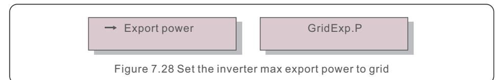
Figure 7.28 Set the inverter max export power to grid
