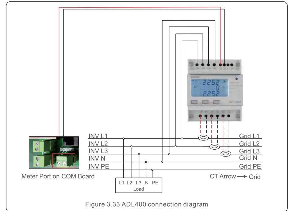
Port 21 of meter connect to meter port A of inverter, Port 22 of meter connect to meter port B of inverter;
