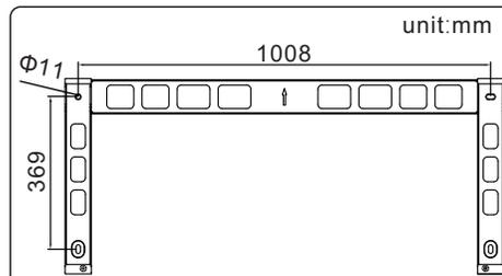
Figure 3.5b Inverter wall mounting (both with AC switch)
