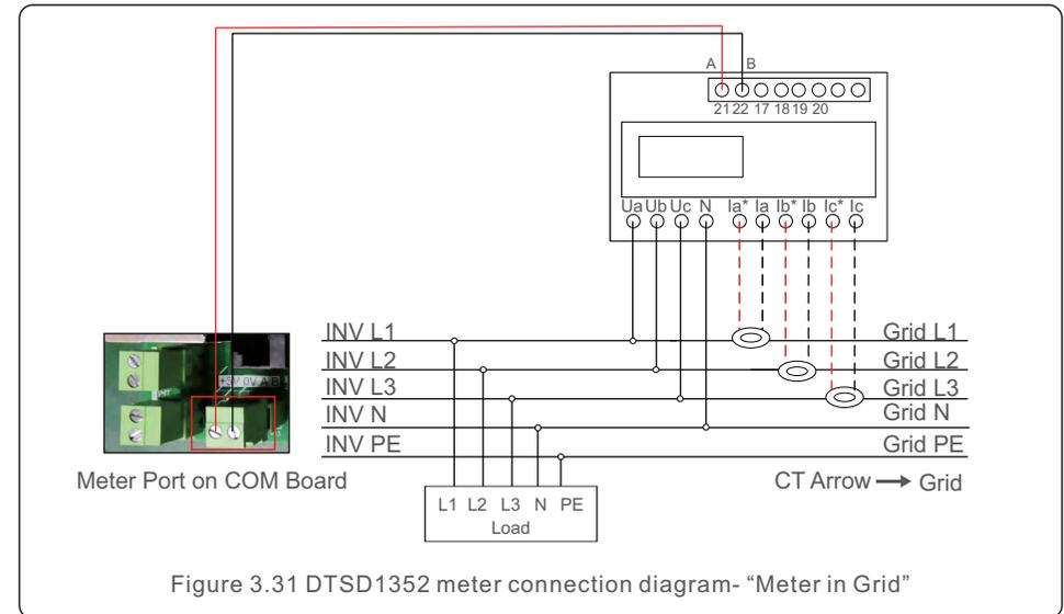
Figure 3.31 DTSD1352 meter connection diagram- "Meter in Grid"
