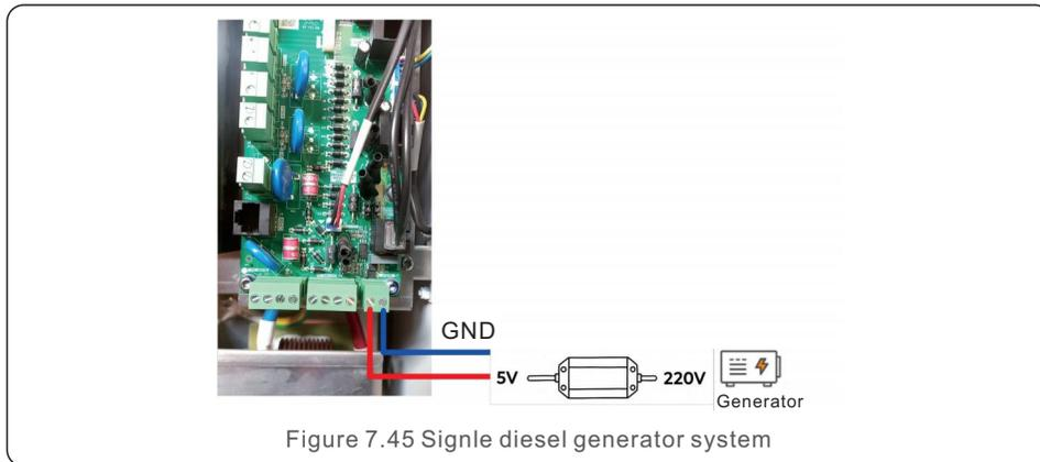
Figure 7.45 Single diesel generator system
