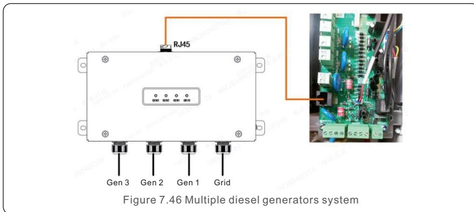
Figure 7.46 Multiple diesel generators system
