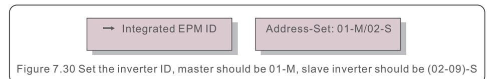
Figure 7.30 Set the inverter ID, master should be 01-M, slave inverter should be (02-09)-S
