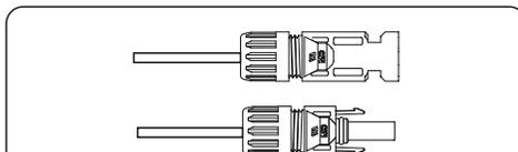
Figure 3.23 Connector with Cap nut Screwed on
