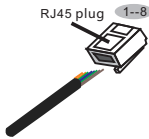
Figure 3.27 Strip the insulation layer and connect to RJ45 plug
