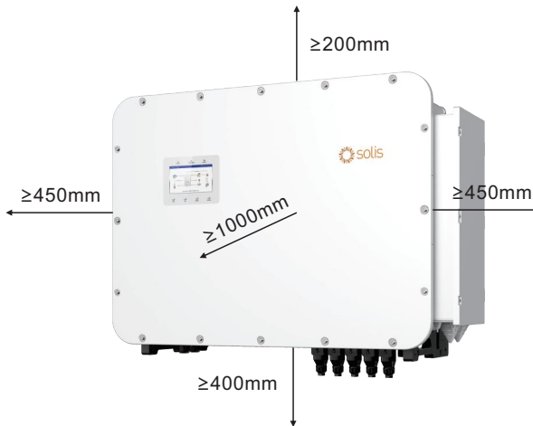
Figure 3.3 Inverter Mounting Clearances
