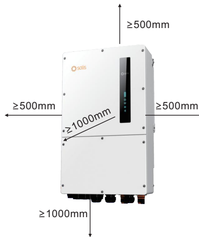
Figure 3.5 Inverter Mounting Clearances
